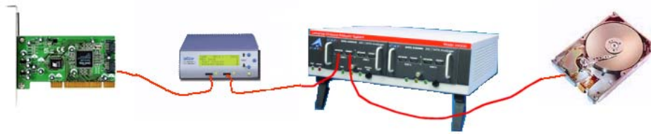
Figure 16 Connection with Analyzer: One-Channel Configuration
