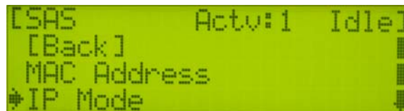
Figure 7 LCD Panel Box Setup Menu: Arrow at IP Mode
