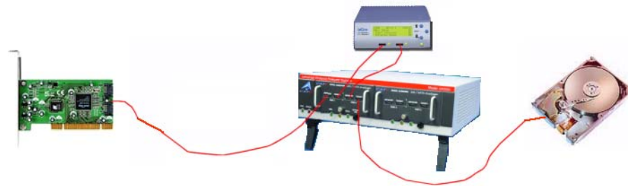
Figure 17 Connection With Analyzer: Two-Channel Configuration
