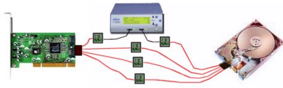
Figure 18 Multiple Connections Using "Octopus" Cables
